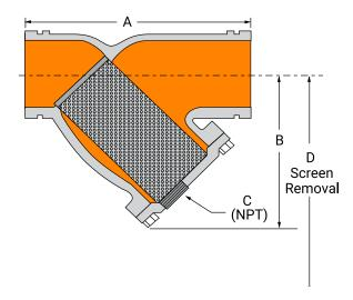
Fig. 758 G Grooved-End "Wye" Strainer
